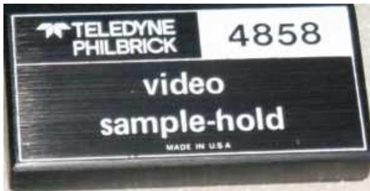
2.5"x5" sample and hold for the 12 bit converter.
